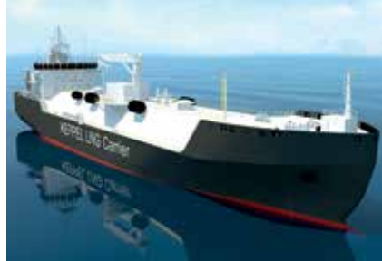
Keppel has designed a range of robust carriers from 3,000m 3 to 30,000m 3 that can deliver LNG along shallow water rivers, coastal areas and inter-islands
